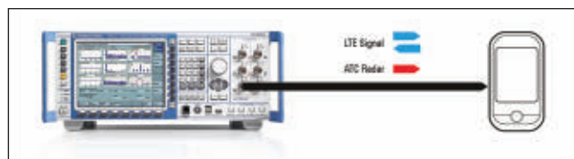
▲ Fig. 4 Test setup for LTE and S-Band radar co-existence tests, using a wideband radio communication tester.
