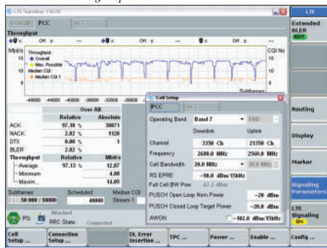
▲ Fig. 8 Modified reference sensitivity level measurement (BLER) while S-Band radar signal is present.
